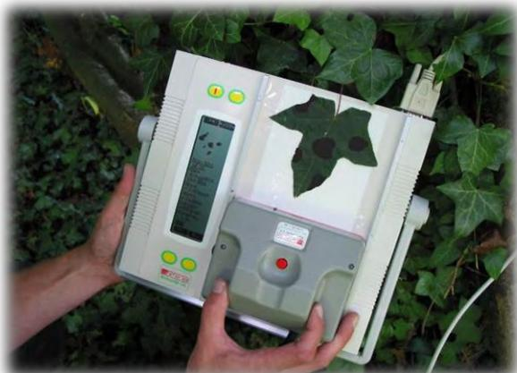
The premier portable leaf area meter with real-time image display for non-destructive, fast measurements and the largest range of calculated parameters (accumulated and mean area, diseased/damaged leaf area, length, width, perimeter, ratio and shape factor). Reliable and robust, with 2 year warranty.
