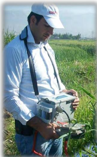
The LCPro-SD [left] is our intelligent, light weight (<6kg) photosynthesis system, enabling full environmental control of variables including CO<sub>2</sub>, H<sub>2</sub>O and temperature.
