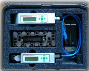
The pocket-sized, easy to use kit comprising a Y(II)/ETR meter for light-adapted 'spot' measurements and an Fv/Fm meter with clips for dark-adaption. All fluorometers listed use Pulse Modulated Fluorescence (PAM) and far red light for full oxidation of PSII.
