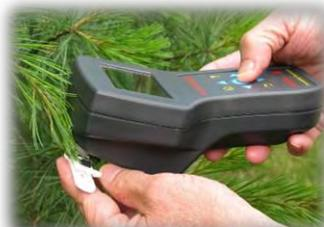
A hand-held, dark-adaption fluorometer for measuring quantum yield, accurate Fv/Fm, Fv/Fo together with advanced OJIP analysis (Strasser et al., 2004) by accurately measuring Fo.
