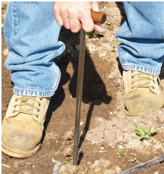
Figure 16 - Coring a hole using the Coring Tool
