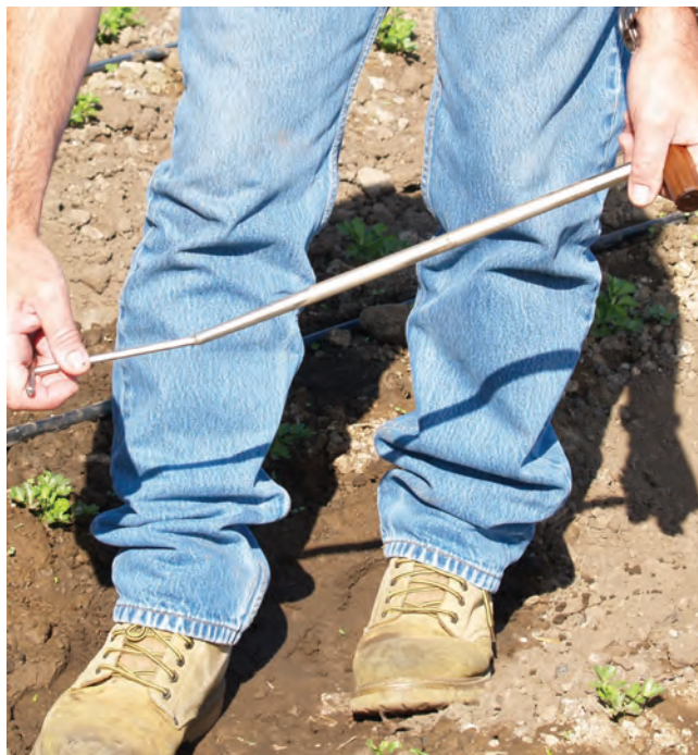
Figure 17 - Using the Cleaning Rod to remove excess soil
