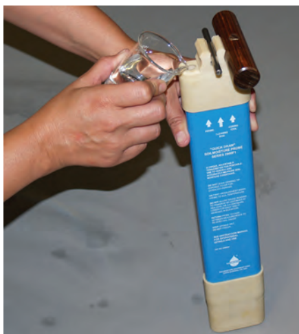
Figure 15 - Filling the probe with water
