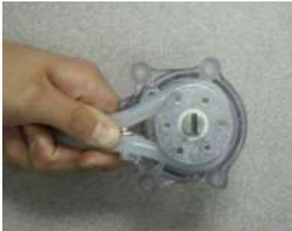
3. Turn rotor counterclockwise until tubing completely surrounds the rotor.
