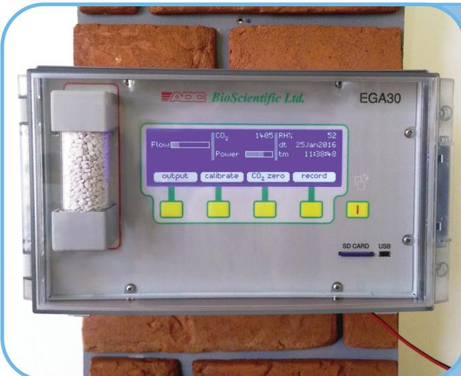
Wall mounted CO<sub>2</sub> Infra-Red Gas Analyser with advanced sensors for water vapour measurement
