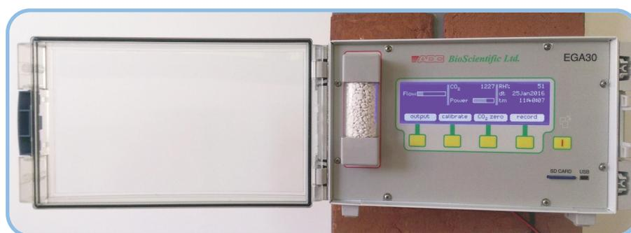
A protective, hinged front panel prevents the entry of dirt, dust and water. It also deters any alterations to the keypad or removal of the memory card whilst measurements are being taken.
