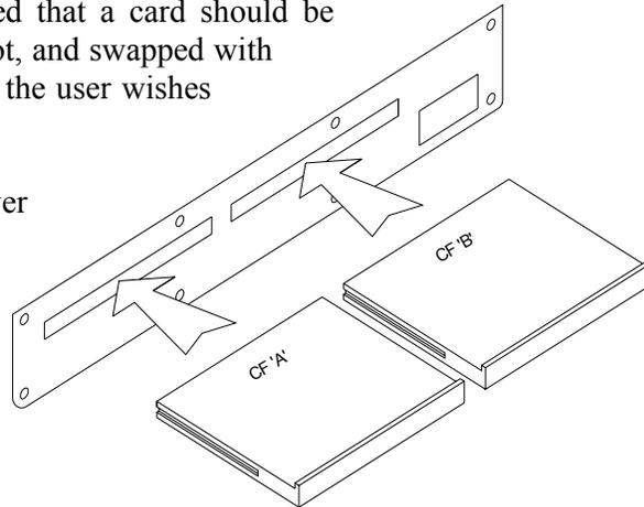
Do not remove a card while the software is accessing it, for example during a format, or when the card's size is being determined just after insertion. If the card has an untimely removal, the software will lock. To restart the processor, press the PAGE key (on the right) and the two left hand keys simultaneously.
