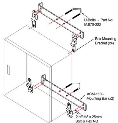
**Setup C - Wooden Fence Post / Wall setup**
