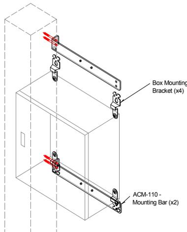
**Setup B - Pole / Tripod mount**
