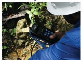
The GPS Aquameter is a hand held device with a display for live data viewing and data recording. As one of our flagship products it is included in every Aquaprobe package. It is designed to be very simple to use and to make your job easier in the field
