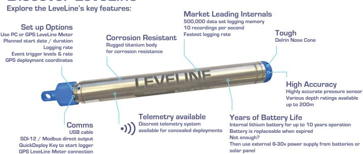
Capture the water level data as quickly as 10 times per second and store up to 500,000 data records on the instrument's built-in memory. All this technology is neatly sealed within a small, corrosion resistant, titanium housing (22 x 186mm) that can be deployed to measure either absolute pressure (ABS, non vented) or gauge pressure (GAUGE, vented) to depths of up to 200m.
