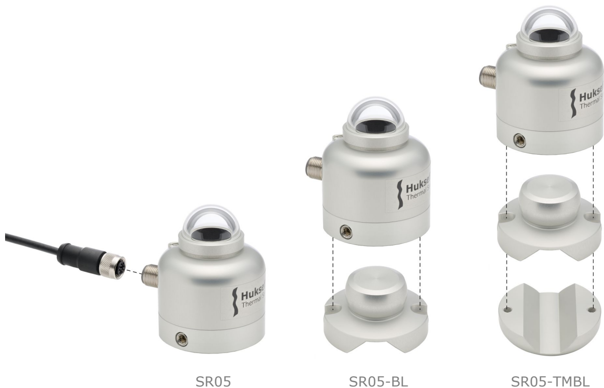
Figure 5.2.1 From left to right: SR05 in its standard configuration with 3 metre cable; with optional ball levelling for easy mounting and levelling on a (non-)horizontal surface; with optional ball levelling and tube mount for easy installation on a 25 to 40 mm diameter tube. Mounting screws are included with the ball levelling and / or tube mount.
