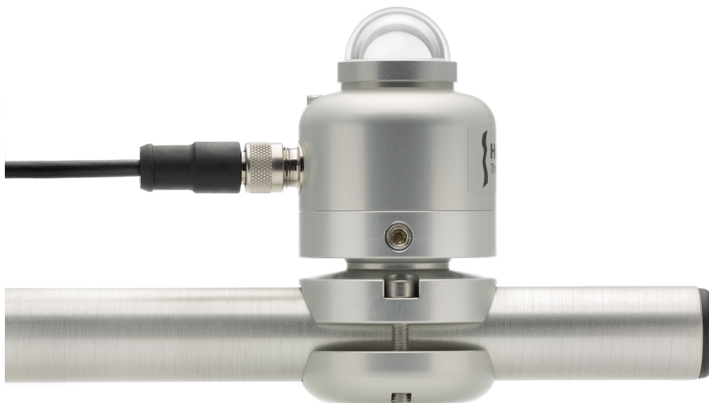
Figure 0.1 On the left SR05-A1 analogue second class pyranometer with bubble level and M12-A cable connector in its standard configuration (3 metre cable standard included); on the right SR05-A1 with optional ball levelling, for easy mounting and levelling on (non-) horizontal surfaces (included mounting screws not displayed)
