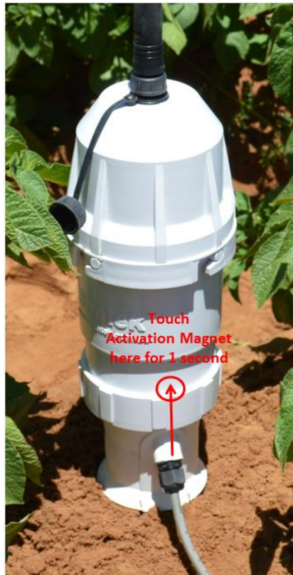
Figure 24 All-in-One Magnet switch position
