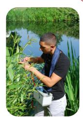
The LCi T instantly calculates and displays a complete set of the most widely utilised parameters for plant gas exchange determination:
