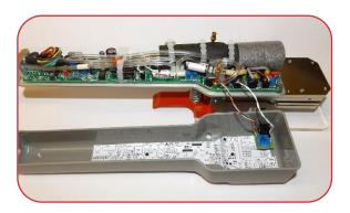
By housing the IRGA directly within the chamber handle, we eliminate any possible response delays in either gas exchange measurements or environmental controls. In addition, this configuration reduces gas 'hang-up' or water vapour 'dropout', which is known to occur in long lengths of gas tubing.
