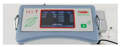
Parameters may be plotted against time or record number, enabling measurement trends to be easily monitored and observed.
