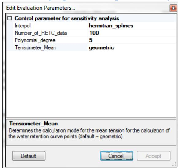
The parameters for raw data interpolation can be edited in a submenu **Edit Evaluation Parameters...** , which pops up when clicking on the respective button on the right side of the header line in register »Evaluation«. The interpolation parameters are described below.
