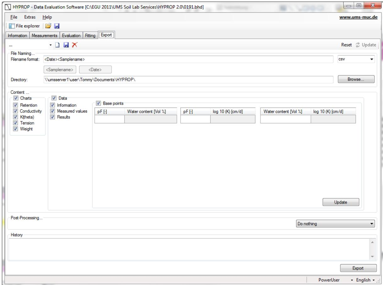
The register “Export” allows the simple export of all graphs, raw data, calculated data, fitted functions, and other parameters of interest.
