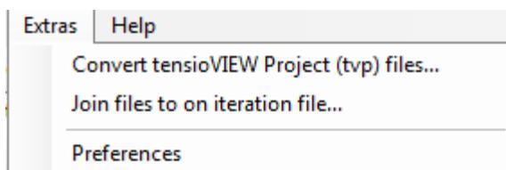
This menu is used to open tensioVIEW projects from HYPROP measurement campaigns, and to combine individual measurements to combined projects. Furthermore, it allows to pre-select preferences for the language and user type, and for the export of data.
