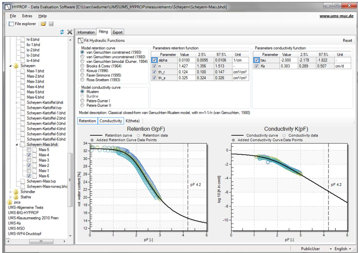
HYPROP-DES offers the convenient and powerful option to assemble individual data sets to combined data sets in so-called HYPROP binary iteration projects (files with extension \*.bhdi). This is of particular use if data sets are to be compared, or if multiple data sets are to be fitted with a single hydraulic function.
