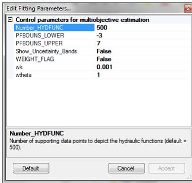
Power Users can edit some of the parameters that specify the calculations and the depiction of the fitted functions. The specifications are listed in the menu “Optimization Parameters” and described below.
