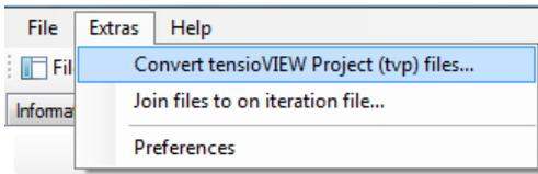
To import raw data from HYPROP measurement campaigns, open the submenu “Extras” and select the option “Convert tensioVIEW Project (tvp) files...”. The imported raw data will be automatically converted to HYPROP binary projects of type \*.bhd.
