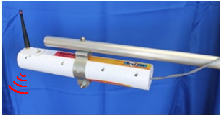
Figure 11: Example of a Correctly Installed SapIP-IRT
