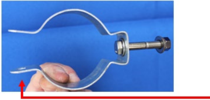
Figure 2: Fastening the SapIP-IRT in Place
